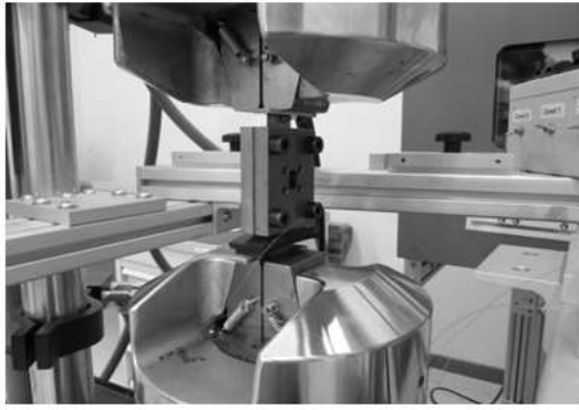
Figure 2. Experimental set-up used in tension/compression cyclic test: a test equipment, b tool for avoids buckling.
